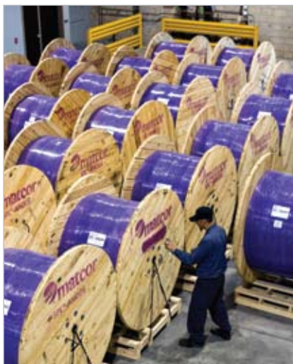
2,500-foot lengths of MATCOR SPL™ Anodes for pipeline cathodic protection.
