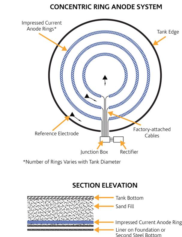
tem prior to field erection of the tank. Once installed and the tank is erected, there is no access or ability to go back and repair the system. A design that eliminates field cutting and welding of the anode and the anode-to-cable connections significantly improves system reliability. With the concentric ring system, all anode segments are factory assembled and tested, with no field connections or welds. This greatly reduces installation time and helps ensure a long, reliable life.
