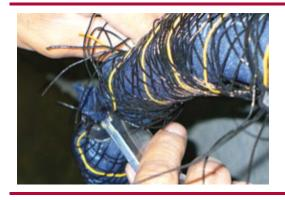
• Using a knife, carefully trim away any excess braiding materials and inert fabric housing. Take care not to damage or cut the insulation of the internal header cable while removing the excess materials.
