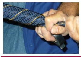
**5**. Tightly compress the coke backfill around the internal header cable and anode assembly.
