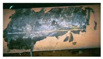
Figure 1. Asphaltic enamel coating failure.
