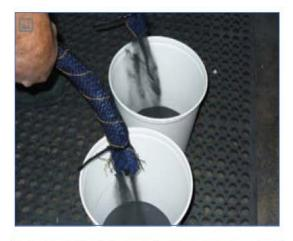
Carefully pour coke backfill from each end to approximately 10 cm (4") of length. Dispose of coke backfill in accordance with acceptable site regulations and requirements.
