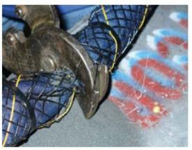
Using an appropriate sized cutting tool, cut completely through the entire assembly, including the anode and internal header cable, yielding 2 separate pieces.
