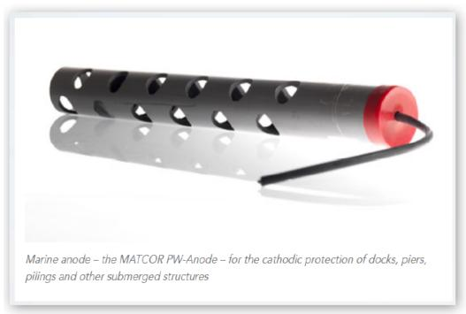
MATCOR's marine anode, the PW-Anode, was developed for the impressed current cathodic protection of structures in marine environments such as docks, piers, platforms, and submerged structures. This anode is also suitable for protecting internal wetted surfaces of process equipment such as aerators, flocculators, clarifiers, digestors, etc.
